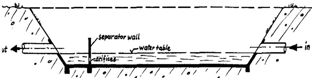
Figure 5-3. Sub-surface fuel separator
