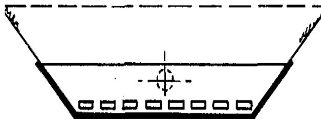
Figure 5-2. Drain water collector with oil separator
