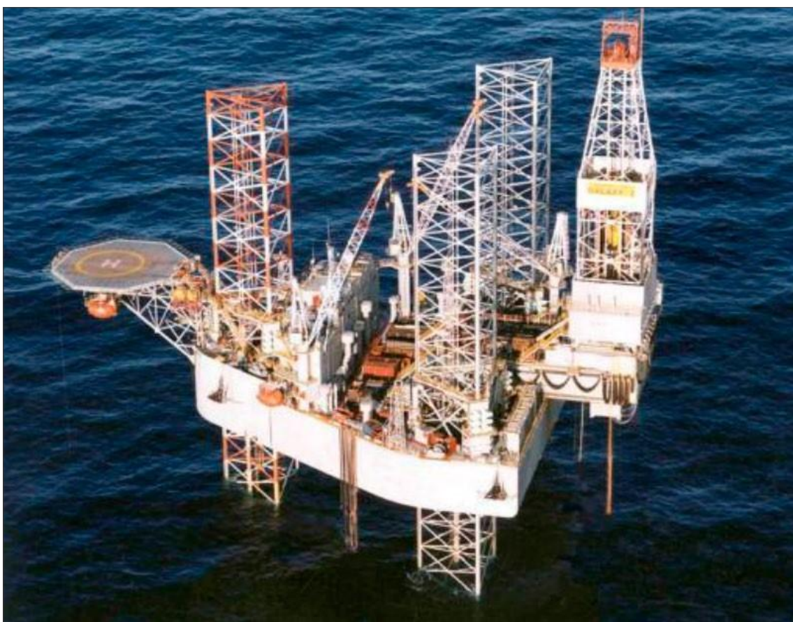
Figure I-1-3. A three-legged jacked-up mobile offshore drilling unit
