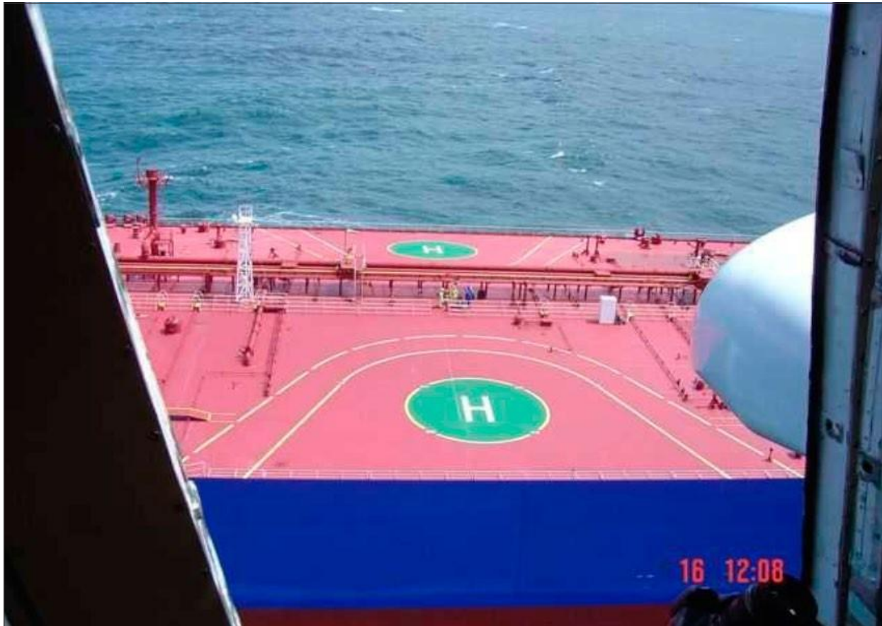
Figure I-1-8. Non-purpose-built ship side landing areas (port and starboard)
