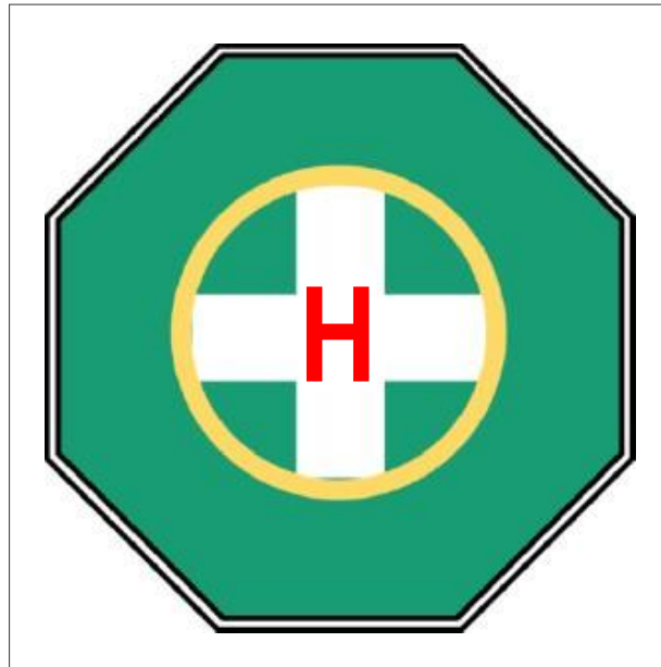
Figure II-5-4. Heliport identification marking with TDPC (hospital)
