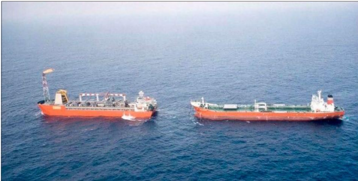
Figure I-1-4. Tanker (right) hooks up with a FPSO (left)
