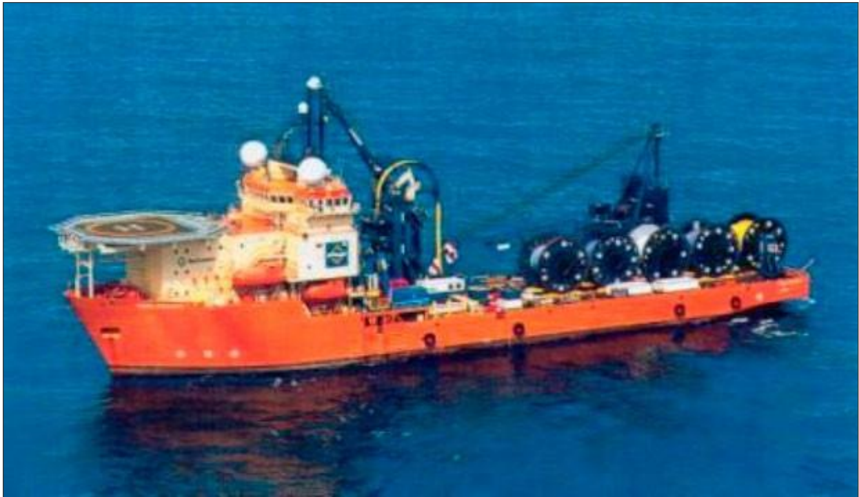
Figure I-1-7. A high bow mounted helideck on a pipe laying vessel
