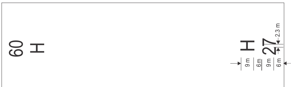
Figure II-5-11. Designation markings for runway-type FATO
