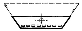
Figure 5-2. Drain water collector with oil separator
