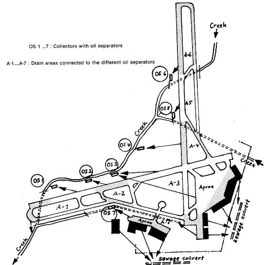
Figure 5-1. Example of an aerodrome drainage system where all drain water from hard surfaces is passed through oil separators
