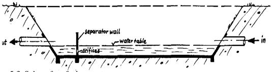
Figure 5-3. Sub-surface fuel separator
