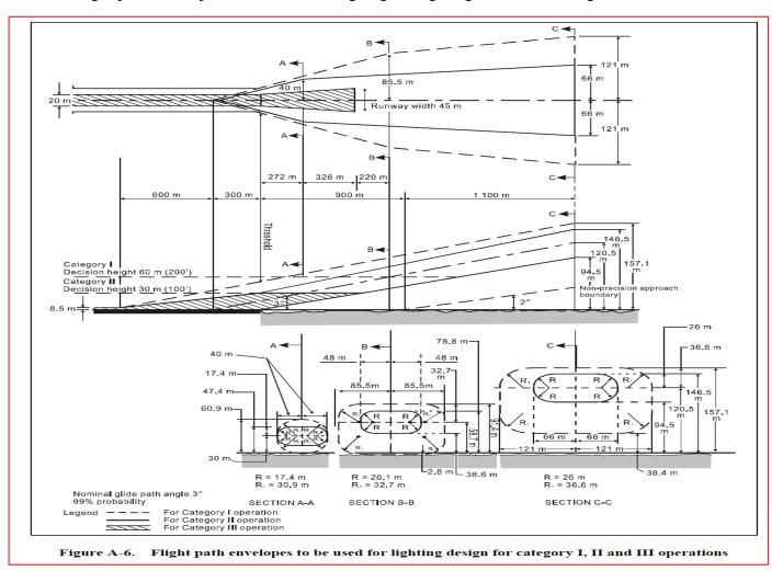
1.3 Flight path envelopes to be used in designing the lighting are shown in Figure A-4.
